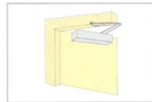
App. 66 Closer fixed to 'push' side of door
